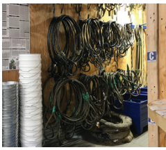
E-track hanger posts for stingers, grounds, air hose whips, and slings
