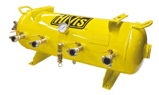
15 Gallon 8 Port HiVis Manifold. Eliminate clutter by running just one air hose to your worksite and connect up to eight pneumatic tools at once. Equipped with a gauge to monitor working pressure and a 200 psi pressure relief valve to prevent excess pressure build-up. Top and bottom brackets allow for easy stacking or mounting to skids or other surfaces. Connect or stack multiple manifolds to handle the busiest worksites.
