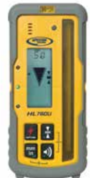
Advanced HL760U Digital Readout Radio Receiver offers automatic Grade Match and PlaneLok (H + V)
