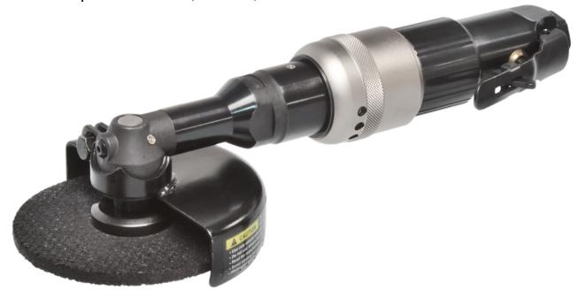
4" Type 1 Extended Angle Die Grinder. 3/8"-24 spindle. Features adjustable side exhaust and a low-profile angle head with 3 position guard for working in hard to work areas. Heavy-duty steel constructed industrial grinders for the toughest applications. Ideal for quickly removing material, deburring, chamfering in shipyards, foundry, welding, petro chemical and fabrication applications. Patented external spindle lock version also available.
