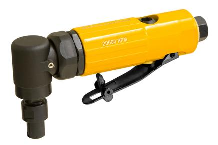
1/4" Collet Right Angle Die Grinder. Features rear exhaust and two-step safety lever. Designed with a hardened alloy steel cylinder and rotor to maintain power while ensuring longer tool life as well as tough alloy steel pinion and bevel gear transmission that is both smooth and quiet. The motor housings are milled from solid aluminum bar stock for precision alignment. Comes with a 1/4" Erikson style collet and two collet wrenches.
